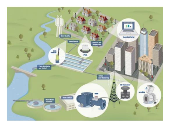
With an AMI network, utilities collect hourly meter reads several times a day. This opens up a whole new set of features that leverage data analytics.
